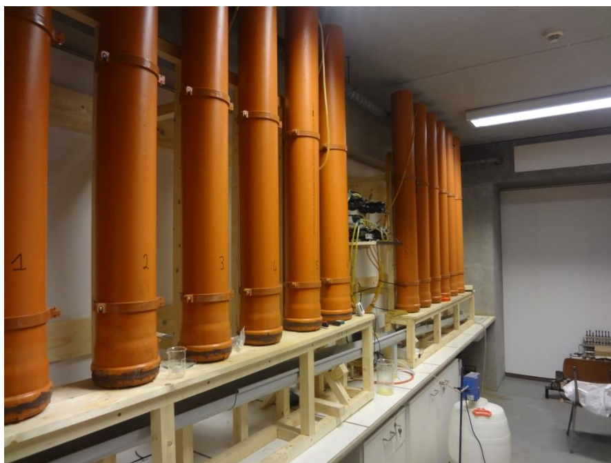
Figure 3: General overview of the oxidation columns: 12 x oxidation columns and associated equipment.
