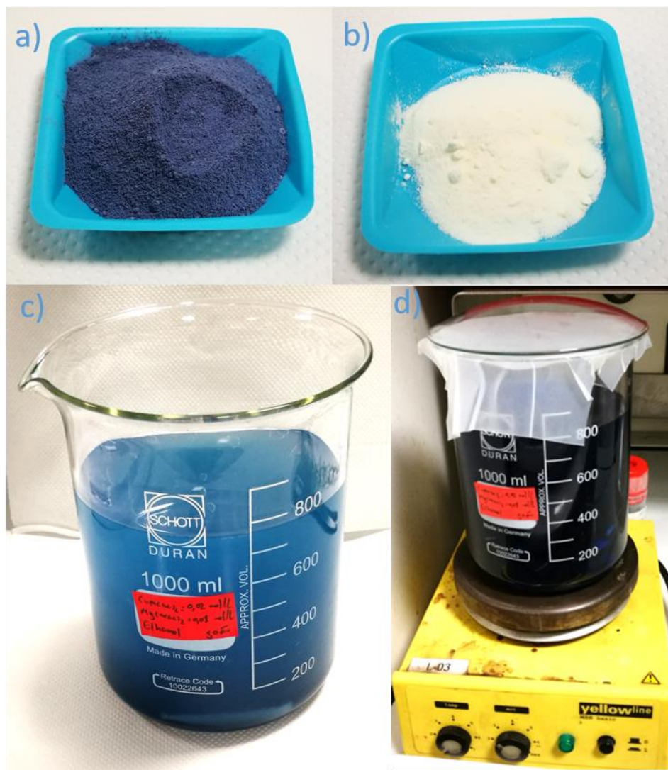
Figure II-22 Precursor used in the solution a) \text{Cu}(\text{acac})_2 and b) \text{Mg}(\text{acac})_2 ; solution after the addition of the solvent; d) stirring step in the magnetic plate.
