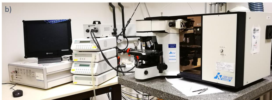
Figure II-35 a) Scheme with Rayleigh and Raman scattering representation 25 ; b) Jobin Yvon/Horiba LabRam spectrometer in LMGP
