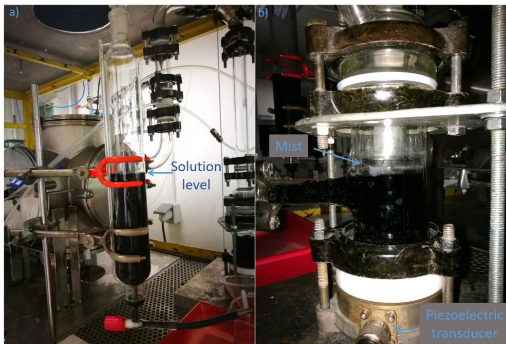
Figure II-25 a) solution vessel with the level of solution visible; b) piezoelectric transducer and created mist.
