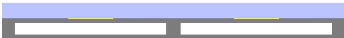
Figure 1.6: Illustration of a 2 by 1 array of 2D CMUTs.
