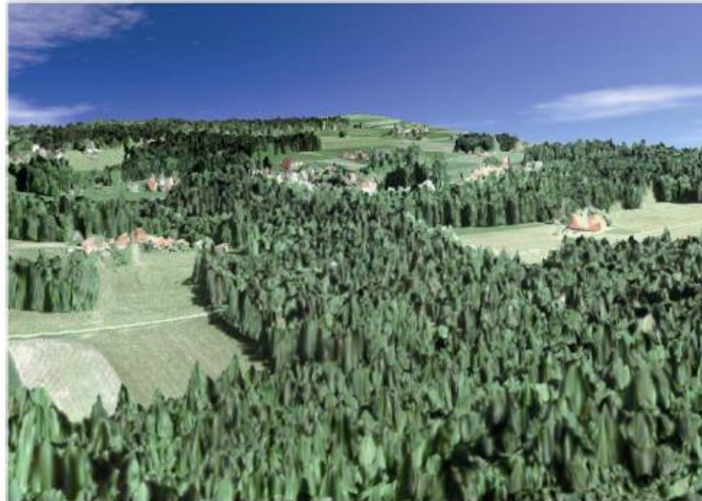
Fig. 3. Forest heights derived from the Pol-InSAR technique overlaid on a Google map from Traunstein, Germany (forest height retrieval based on two fully-polarimetric L-band data sets acquired by DLR's airborne E-SAR system).
