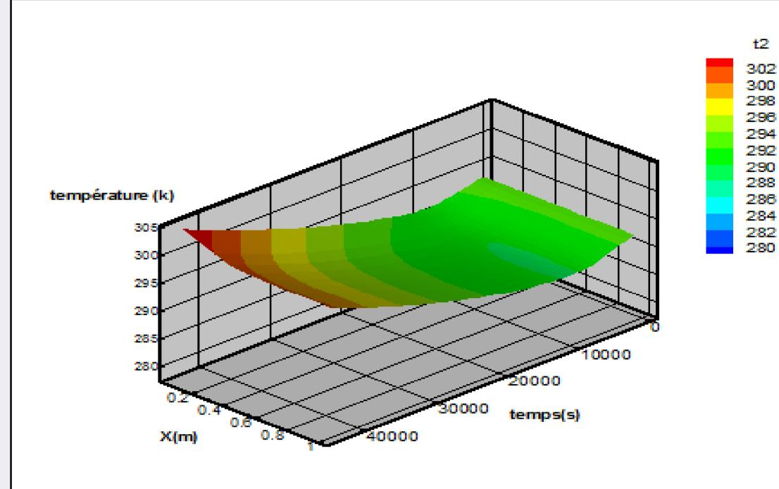
Evolutions of the internal heat transfers inside the mortar during drying.
