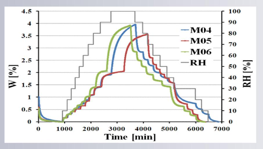
Changes in moisture content of mortar M04, M05 and M06 with the variable RH levels over the time during isotherm sorption runs at 20°C
