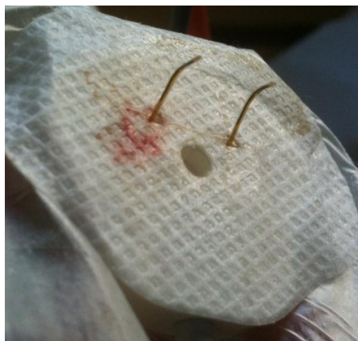
Figure 3.2 The underside of the Sentrino sensor. The two filaments are inserted in to the subcutaneous layer with the help of two hollow retractable needles that encase the filaments.
