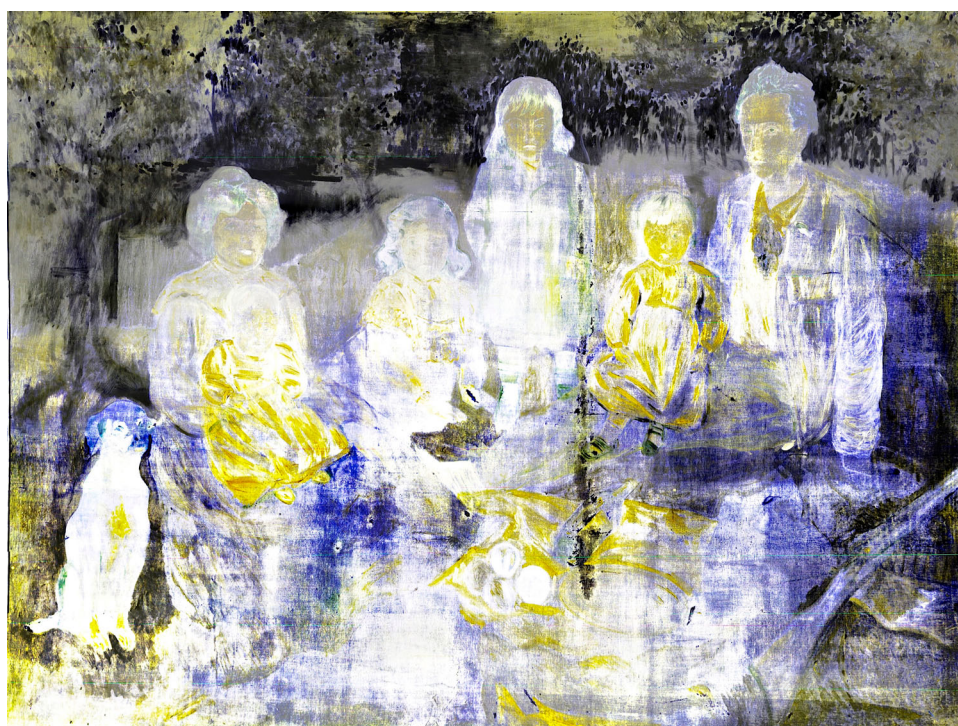
Figure 6. Infrared hyperspectral image acquired with a Specim SWIR camera, providing spectral information from 1000 to 2500 nm and using pushbroom mode. Colors correspond to intensity at 1100, 1500, and 2000 nm.
