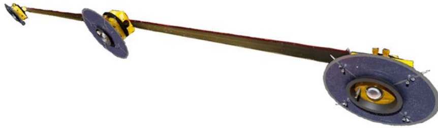
Fig. 1. Overview of the Pegase space-based interferometer. The two siderostats are flying in linear configuration with the beam combiner spacecraft located in the middle of the formation.
