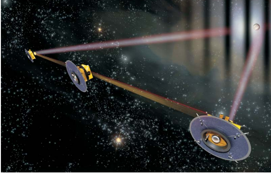
Figure 3.4: Overview of the Pegase space-based interferometer. The two siderostats are flying in linear configuration with the beam combiner spacecraft located in the middle of the formation.
