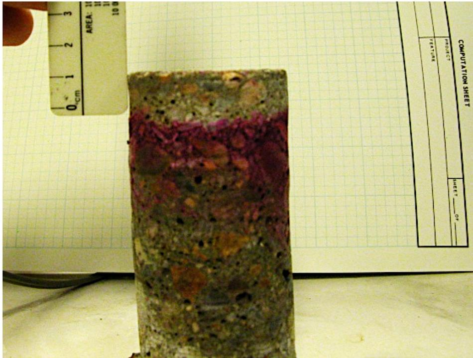
Figure 0-2: Carbonation depth measurement on a freshly exposed concrete section using phenolphthalein
