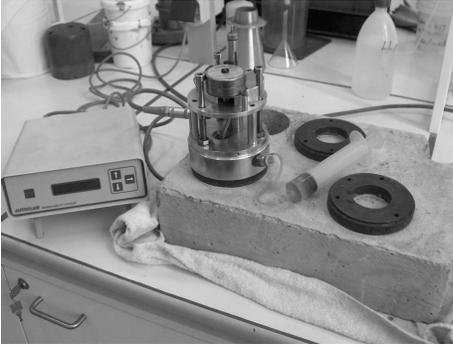
Figure 5-2: Autoclam system and electronic controller
