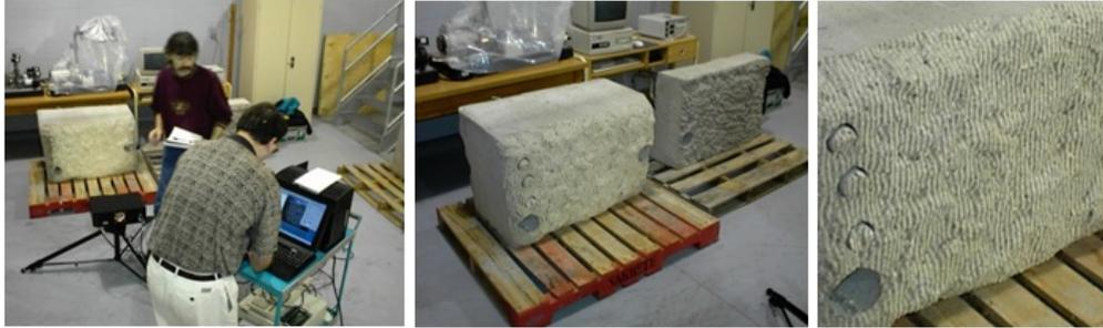
**Figure 2-18: Use of an interferometric measuring device for concrete surface characterization**
