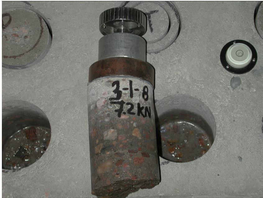
**Figure 0-11: View of a 4°-inclined core after pull-off extraction**
