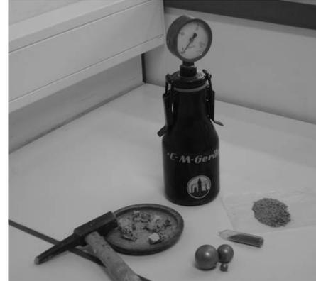
**Figure 5-6: Carbide bomb test**
