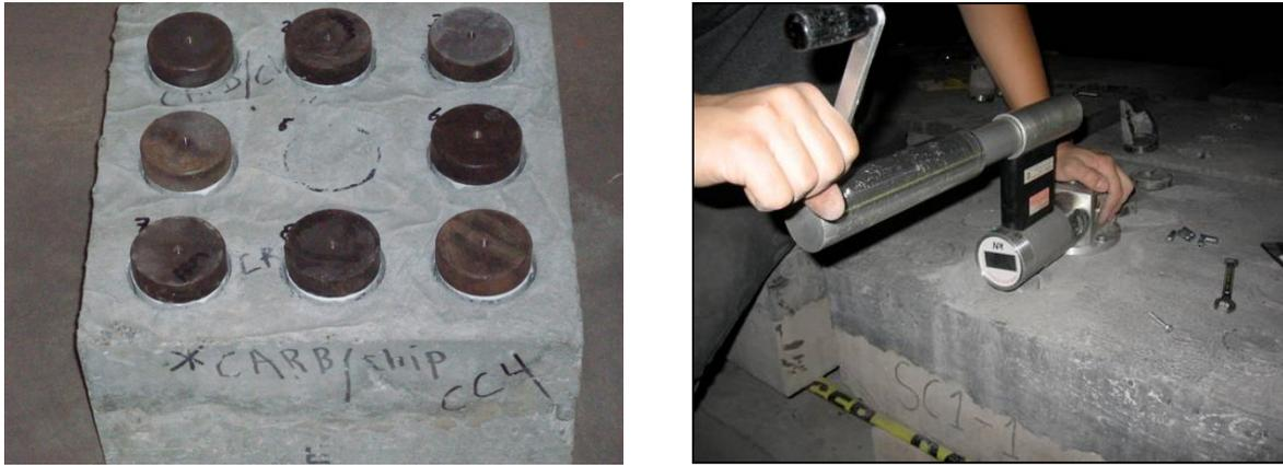
Figure 0-4: Pull-off bond test apparatus
