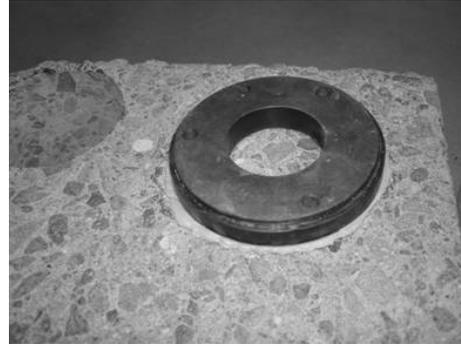
Figure 5-3: Gluing of the ring onto the concrete substrate (ISAT)
