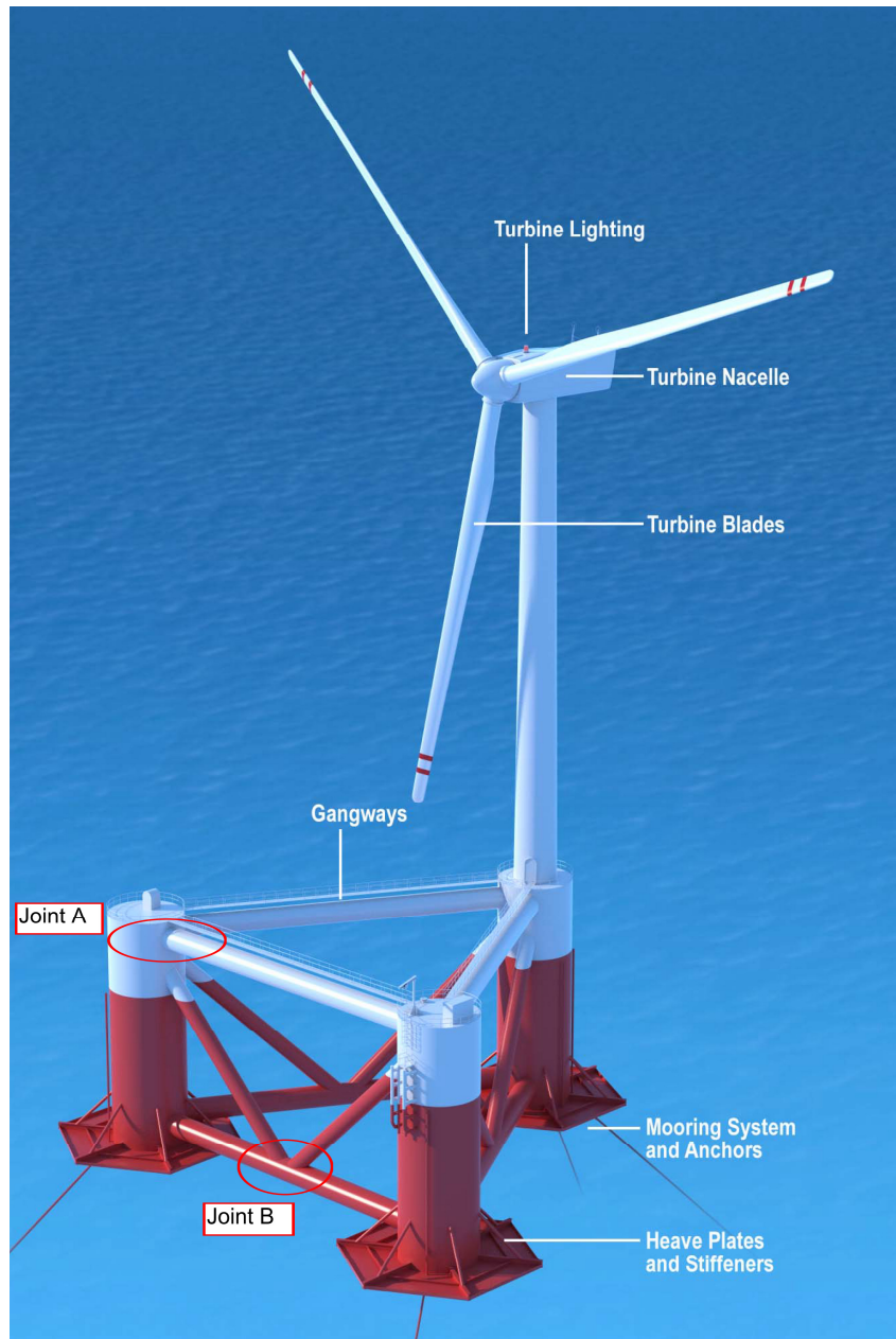
FIGURE 4.1: Position of Joint A and Joint B in a floating offshore wind turbine (source: Wikipedia)
