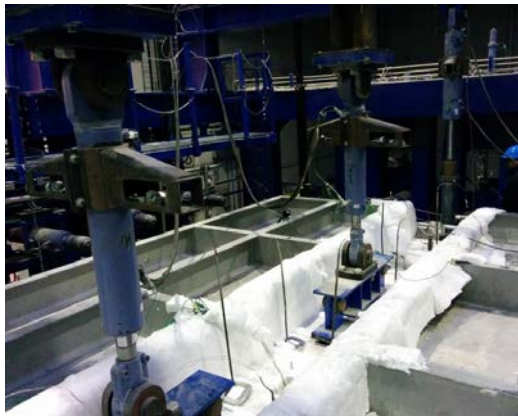
a) The setup of the beam outside the furnace
