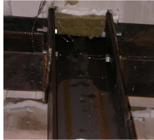
Figure 3-4 : Geometry of the tested double-sided joint with flush end-plate connections
