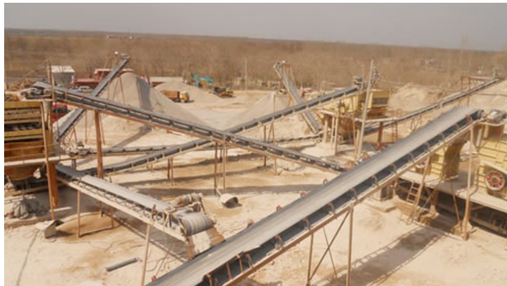
Figure 6.1: (From XSM mining and construction) Photography of a gravel sand production line. The granular material is transported by conveyor belts and vibrating screens through the different production stages.
