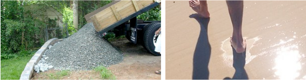
Figure 1.2: (Left) A heap of gravel can naively be compared to a granular solid. While pouring, a particular angle of repose is obtained. (Right) The pressure of the foot on the sand creates a dry zone by absorbing the water into the pores between the grains.
