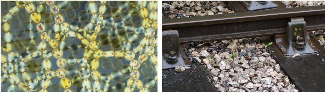
Figure 1.4: (Left) Picture obtained by exerting pressure on stress birefringent particles. The highlighted zone correspond to the force network through the granular media. (Right) Ballast used to prevent rails from sinking into the ground.
